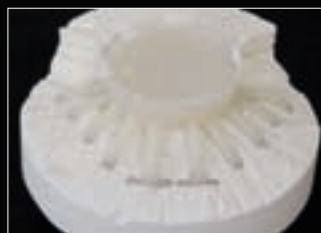
Figs 7a and b: Before the pressed objects are entirely divested, the press sprues have to be separated. This eliminates tensions which might occur during the cooling of large press cones.
