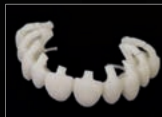
Figs 7a and b: Before the pressed objects are entirely divested, the press sprues have to be separated. This eliminates tensions which might occur during the cooling of large press cones.
