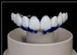
Fig. 6: The press sprues are attached at an angle between 45° and 60° using the 300 g investment ring of the IPS InLine PoM system.
